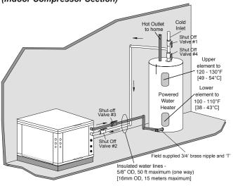
Figure 16: HWG Double Tank Installation (Indoor Compressor Section)
